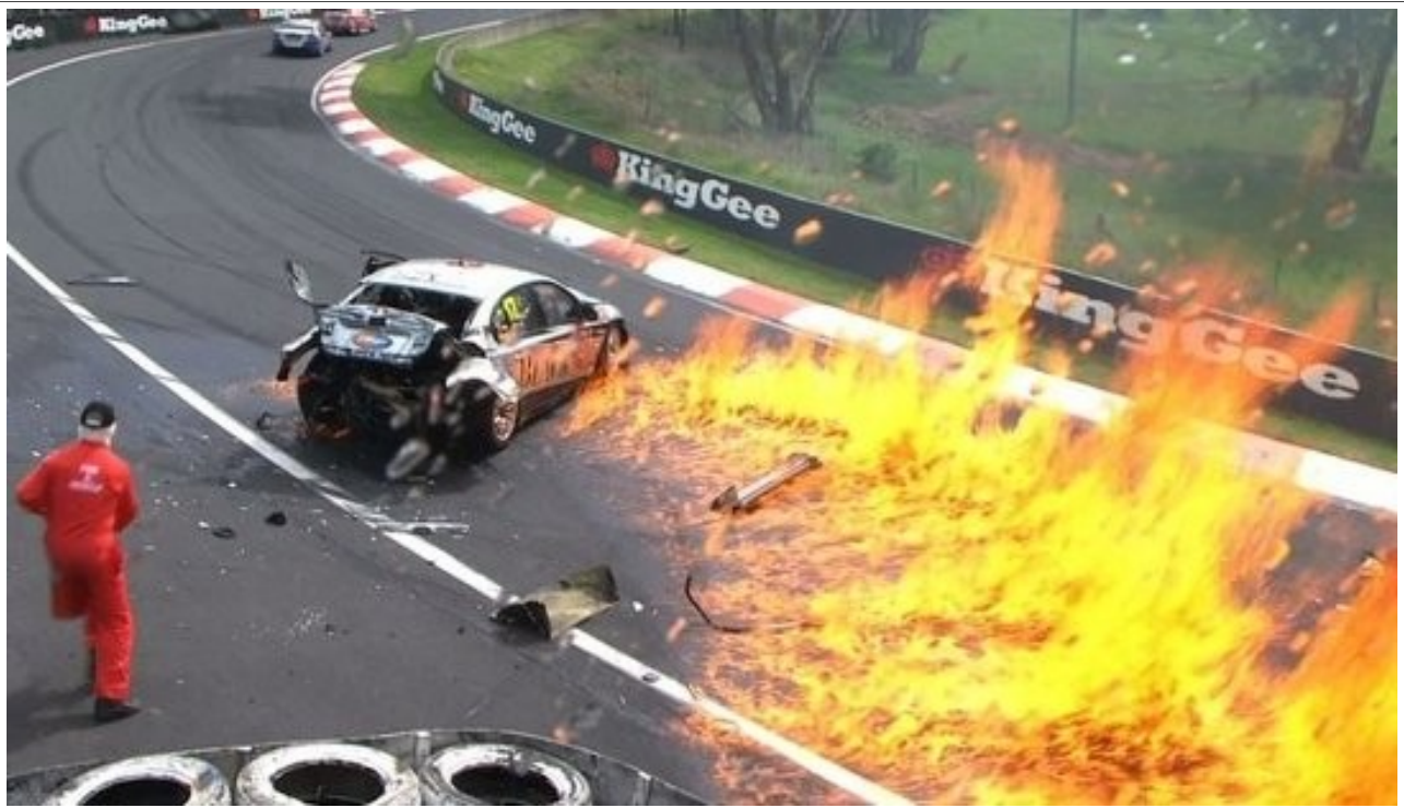
David Besnard leaks fuel which catches fire after he struck the wall at Bathurst with his rear left quarter panel, rupturing the fuel bladder. Two fire marshals were quickly on the scene to douse the flames.
